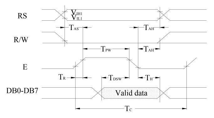
•Reading data from ST7920 to MPU
