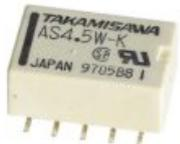
Typ AS4.5W-K Spule: 4,5V-/145 Ohm monostabil, 2-polig UM 30V/2A. Maße (LxBxH): 14x9x6 mm. Pos.N4320 nur..... €-,75
